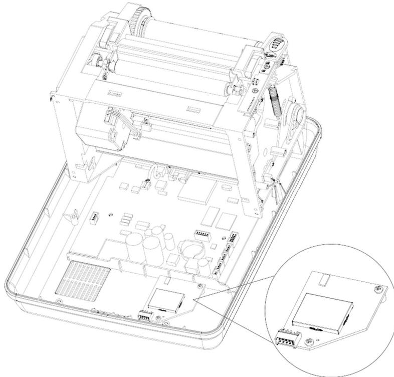
3. Plug the Bluetooth cable to **J15**, which is the black port located to the lower-right of the main board. Route the Bluetooth cable outside (right) of the row of connectors.
