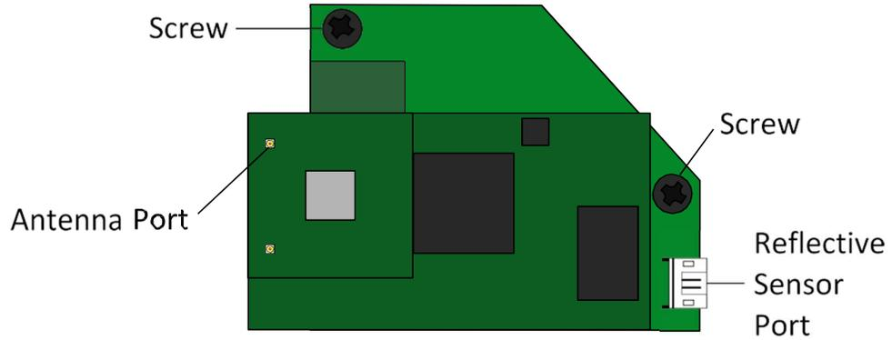
2. Below the main board, you'll find two screw holes on the lower-right. Align the two holes on the Wireless LAN card with them and secure the card with two screws.
