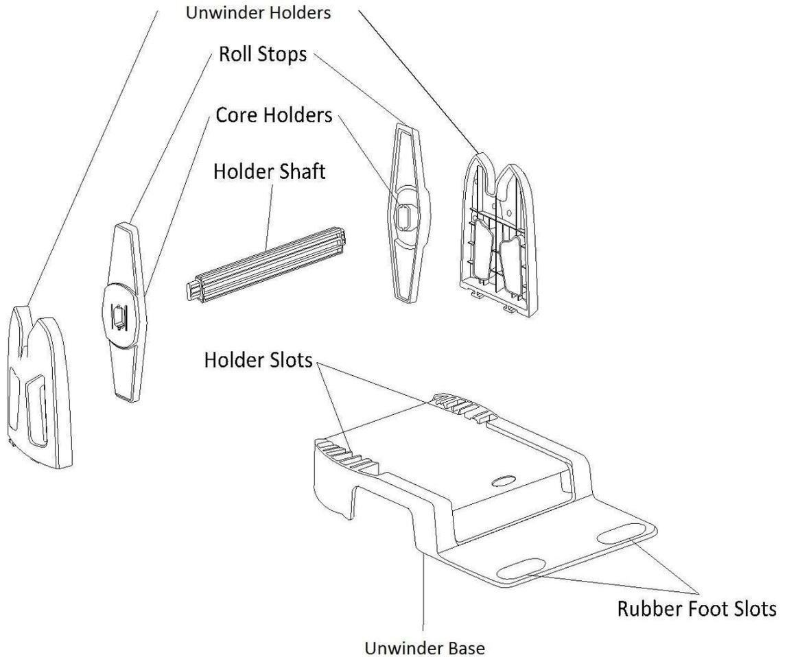
To install an external unwinder:
