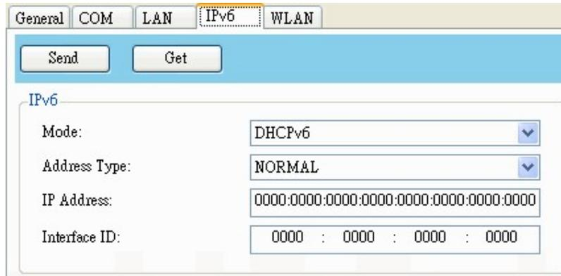
2. After your printer restarts, click **Get** to get its IPv6 information. If you are using a static IPv6 address, you'll get the same settings as it is in the previous step; if you are using DHCPv6, the DHCPv6 server will automatically populate the **IP Address** and **Link-Local Address** boxes under **Current IPv6**.
