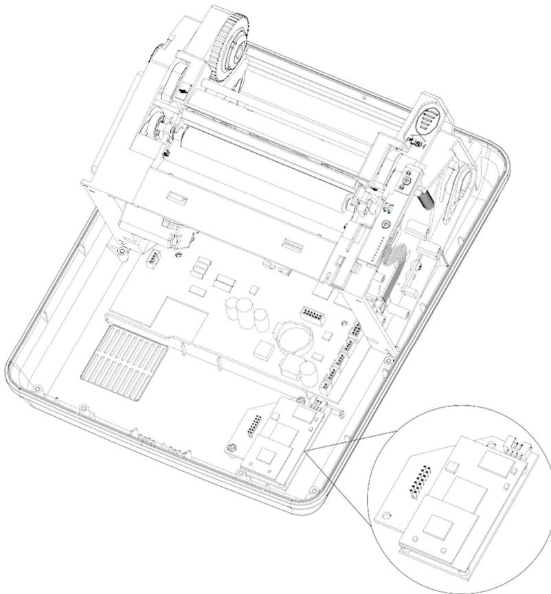
3. Plug the Wireless LAN cable 1 (white connector) to **J13**, which is the white port located to the lower-right of the main board.
