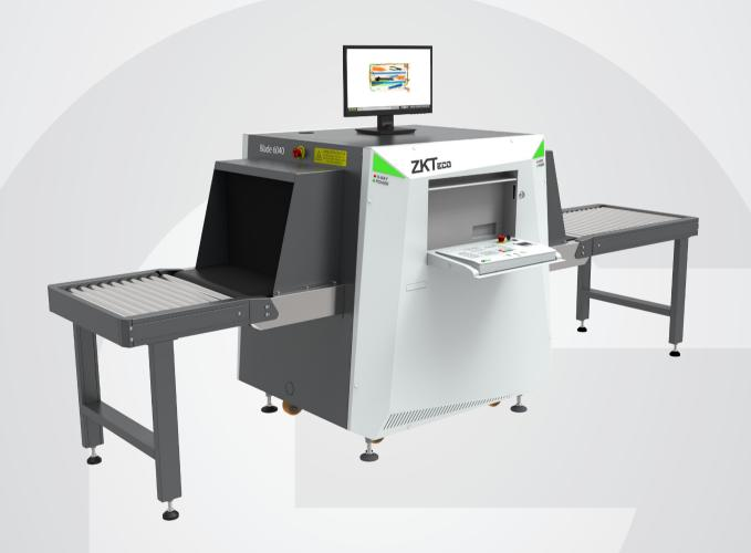
BLADE6040 is a X-ray baggage inspection which has a tunnel size of 610 mm by 420 mm and can provide the effective inspection of mail, hand-held baggage, luggage and other items. It allows identification of weapons, liquids, explosives, drugs, knives, fire guns, bombs, toxic substances, flammable substances, ammunition, and dangerous objects, which are safety hazard by identification of substances with effective atomic number.
